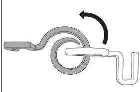
3 Put Tip of Hook B onto Tip of Hook A, just like shown in below. And slide Hook B toward to Hook A with pushing backwards.
